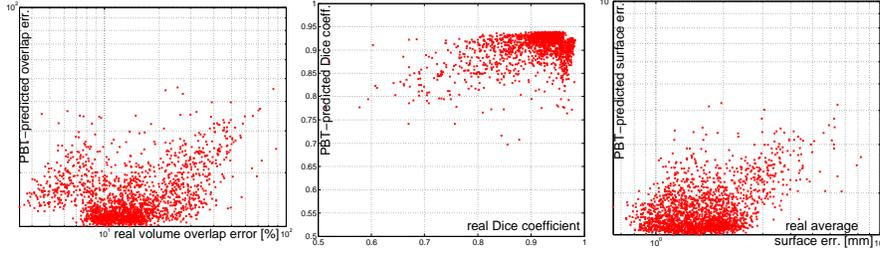
**Fig. 2.** Real segmentation errors (x-axis) versus linearly regressed PBT-probabilities (y-axis). Correlations coefficients (left to right): 0.45, 0.48, 0.49. Max. surf. err.: 0.29. (Note that for readability we have adopted linear and log scaling where appropriate.)
