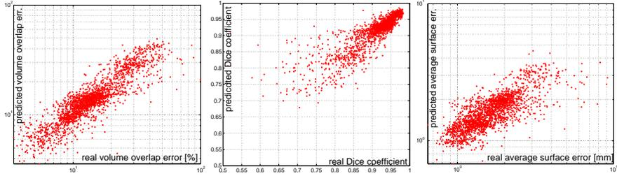
**Fig. 3.** Real segmentation errors (x-axis) versus SVM regressor-predicted ones (y-axis). Correlations coefficients (fr. l. to r.): 0.85, 0.79, 0.56. Max. surface error: 0.69.
