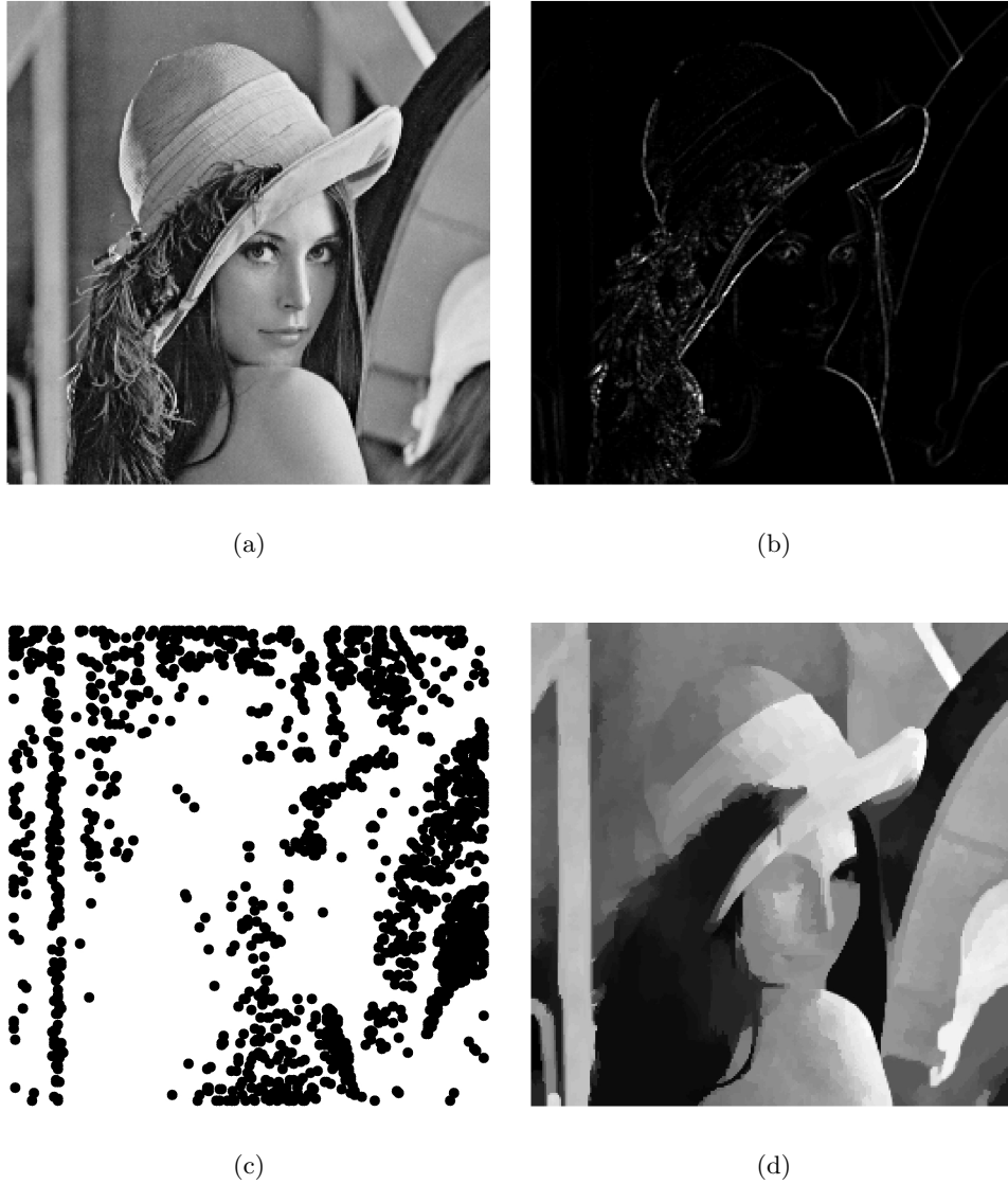
Figure 7.4: Anisotropic interpolation of an image based on very sparse sampling. (a) Original Lena image. (b) Magnitude of image gradient. (c) Samples taken from lowest magnitude points. (d) Anisotropically interpolated image. \beta^1 = 95
