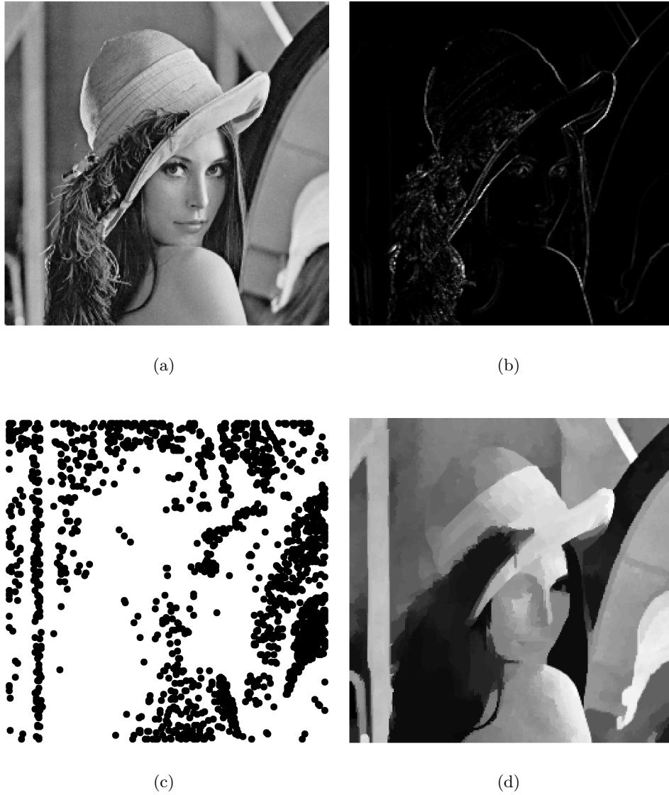
Figure 2-11: Anisotropic interpolation used to low-pass filter an image. (a) Original Lena image. (b) Magnitude of summed image gradients. (c) Samples taken from lowest magnitude points. (d) Anisotropically interpolated image.
