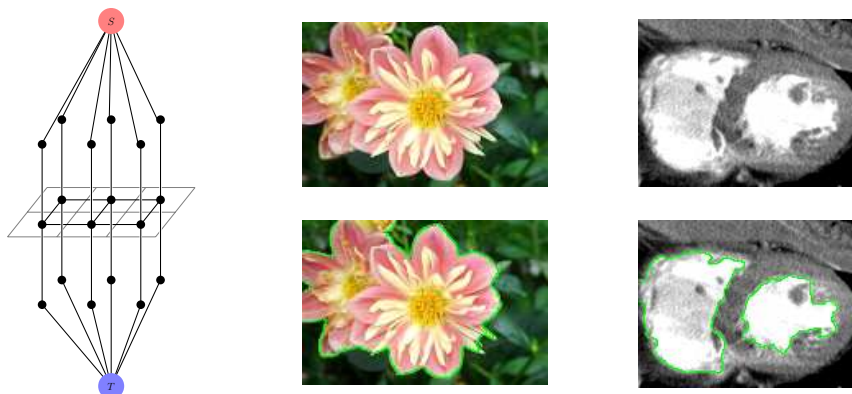
FIG. 4.6. Example of graph construction to incorporate unary terms for unsupervised segmentation. Each node is connected to a source node and sink node through an intermediary node which is weighted to reflect the strength of the positive and negative unary term. This construction is then applied with a simple appearance prior to automatically segment two images.
